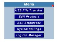
All the Menu options except **Change Manager** will be locked out after 1-minute of screen inactivity for all Managers with Admin capabilities. This does not apply to the "Master" user described in Section 3.
