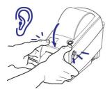
**4:** Close the printer. Gently swing the top cover down onto the printer's base. Press down on both sides until the cover snaps closed, typically with an audible sound.
