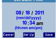
will be grayed out. Pressing the button displays the **Set Date/Time** adjustment screen. Touch the blue numbers to enter the date and time. Touch the blue date format to toggle: mm/dd/yyyy, dd/mm/yyyydd-mm-yyyy
